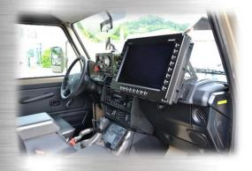
Computer system (2 computers and 3 monitors) with user friendly software interface enables instrument use, control, data and alarms visualization and CBRN reporting (ATP-45). Radio station (HF and VHF) enables transmission of data and speech.
