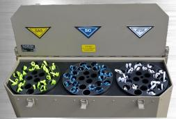
Automated marking system is intended to mark the area where any danger has been detected. We use flags to warn others of possible danger in this area. The marking system is usually installed on a reconnaissance vehicle, which marks the area with flags when danger is detected. Flags can be released during slow driving.
