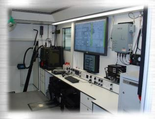
Chemical analysis with Mobile Mass Spectrometer, air-surface probe, gas chromatograph and surface sampler provides identification capability from any medium (soil, water, air). Biological detection enables automatic start of air sampling for further PCR analysis inside glove box.
