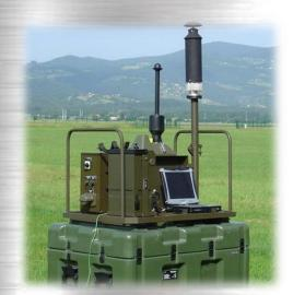
Stand Alone Unit consists of two cases. A battery is integrated in the power supply case and takes care for autonomous operation of the unit.
